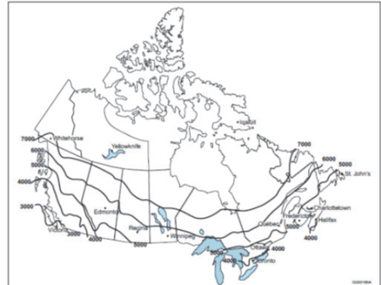
NECB 2015, Appendix Figure A-1.1.4.1.(1) – Contour Map of Approximate Annual Heating Degree Days
